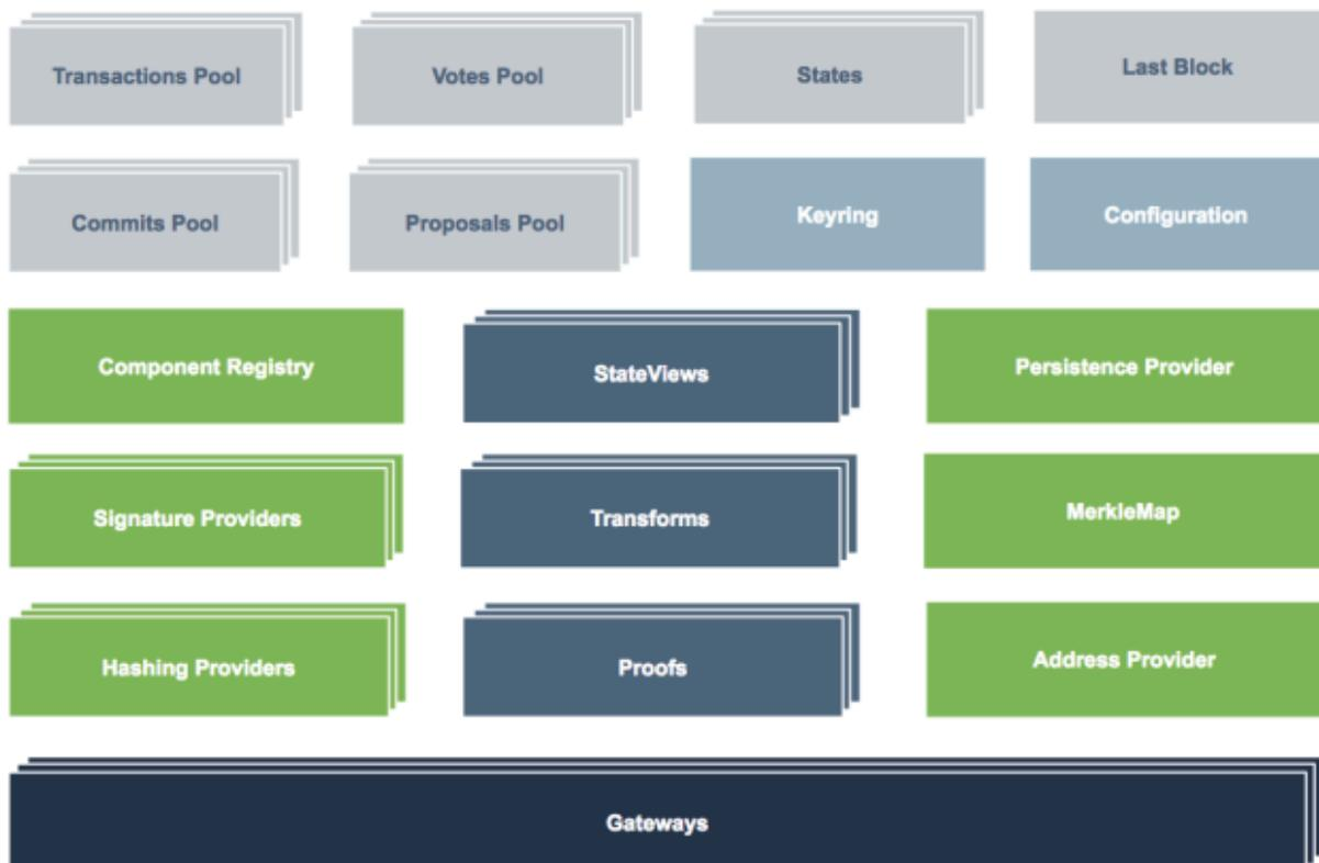
Largely speaking, the system is divided up in that the grey boxes are consensus primitives, the green boxes are cryptographic and systems integration primitives, and the blue boxes are user land.
